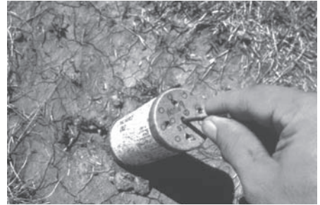
Figure 8. Insert the fuse deep into one of the center holes but with enough fuse extended to insure safety.
