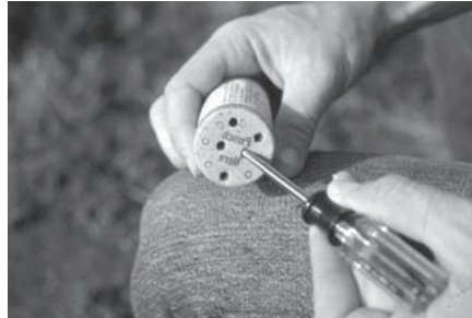
Figure 7. With a nail or Phillips screwdriver, punch several holes about 1/2 inch in diameter into the designated end of the cartridge. Rotate the nail with each punch to loosen the contents.
