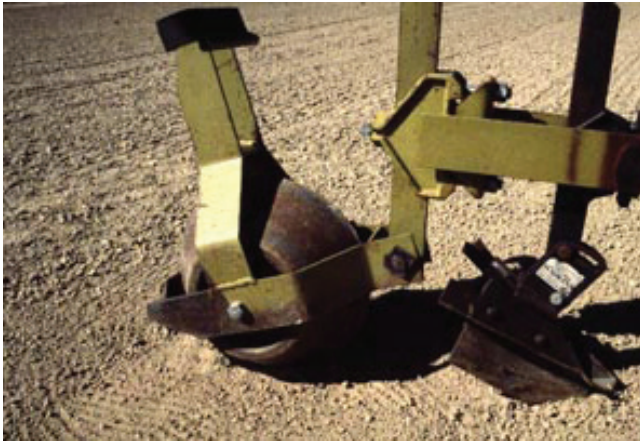
Figure 1. Eversman v-wheel used in Nebraska study.
