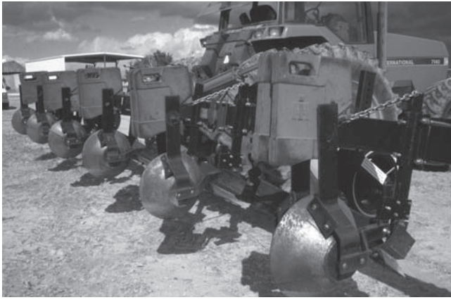
Figure 5. A 12-row furrow opener and firming wheel system.
