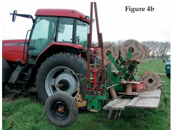
Figure 4a-b. Equipment used to install an SDI system.
