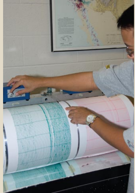
Figure 8. Seismographs, such as this one located at Indiana University, record the waves generated by an earthquake. By analyzing the data on the seismograms, scientists can determine how far away the earthquake occurred and how strong it was.
