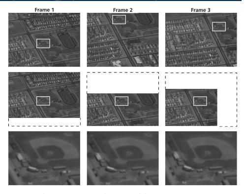
Above, three frames shot successively from an aircraft flying above Albuquerque, N.M., in turbulent weather. The top row shows the raw video imagery with severe camera jitter; the center row, the three frames registered to the same position relative to the baseball field; and the third row, a smooth video stream of the same field in real time.
