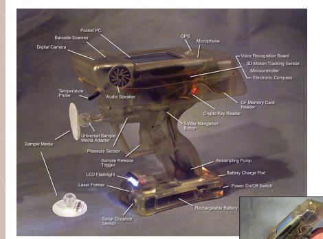
The Hands-Off Sampling Device's unique combination of sensors, tracking systems, and recording devices—coupled with its ability to take a wide variety of samples—makes it the ideal tool for doping testers at sporting events such as the Olympics, border inspectors, first responders, archeologists, crime-scene investigators and forensics personnel, waste and weapons inspectors, and ecologists.
