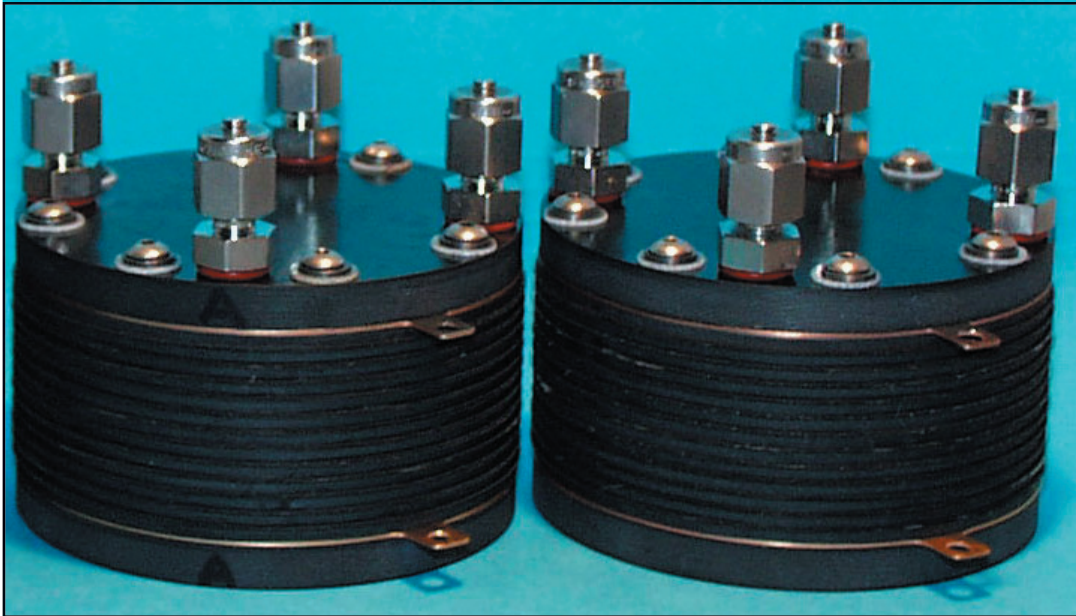
A pair of Los Alamos stacks used in the DMFC-20 power system
