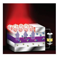
LANL's quantum dot portfolio includes a high-efficiency light emitting diode (LED) design based on non-radiative energy transfer from a quantum well into a layer of colloidal quantum dots.
