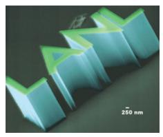
LANL's Energetic Neutral Atom Beam Lithography/Epitaxy technology (ENABLE) provides selective etching of polymers with sub-100 nm features and aspect ratios of up to 35:1. ENABLE promises to open new frontiers in precisely defined nanoscale polymer structures and optofluidic interfaces.
