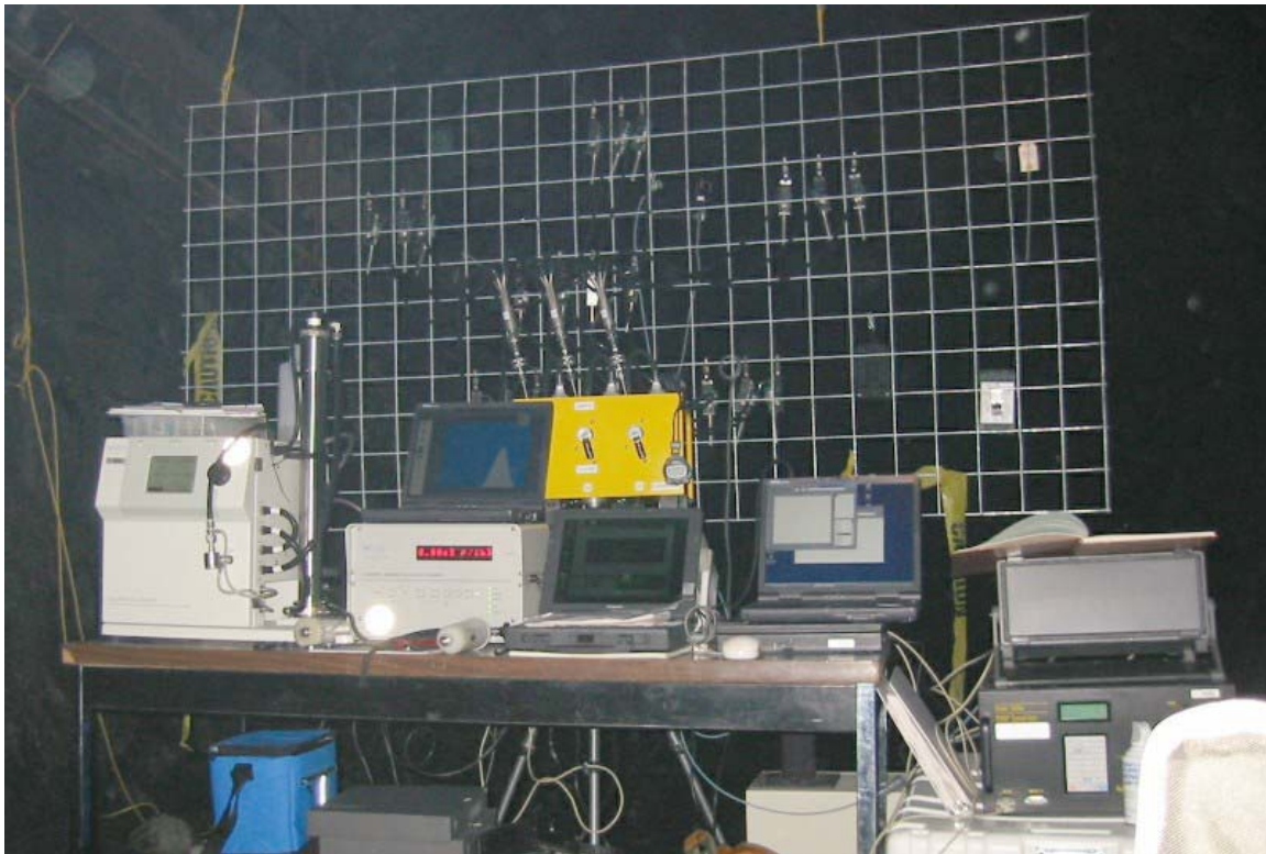
Figure 13. Downstream sampling station showing instrumentation and grid supporting DPM samplers, anemometer, iTX gas monitor
