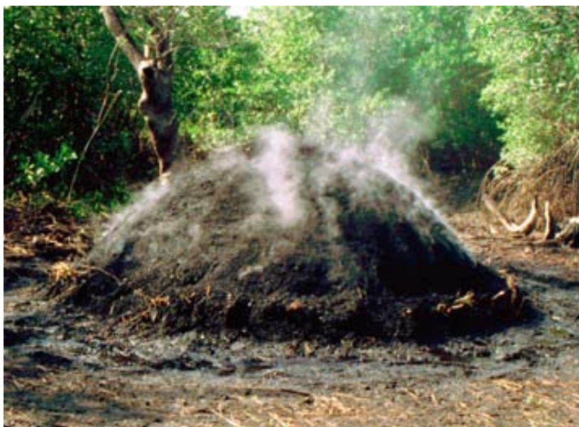
Top: Charcoal treatment plant established with the DANIDA Mangrove Project in Pacific Costa Rica, supported by IUCN and CATIE. Bottom: Typical earthen kiln used to convert stacked red mangrove poles into charcoal for local heating needs, Pacific Panama. PHOTOS: N.C. DUKE
