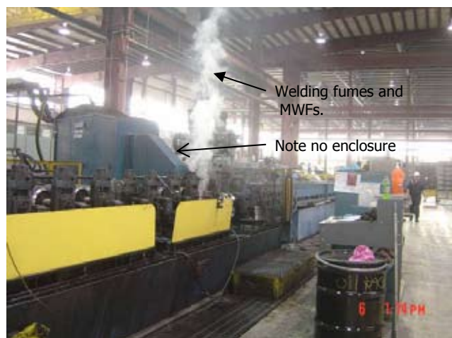
Photo 1: Mill forms conduit out of sheet metal and welds the seam
