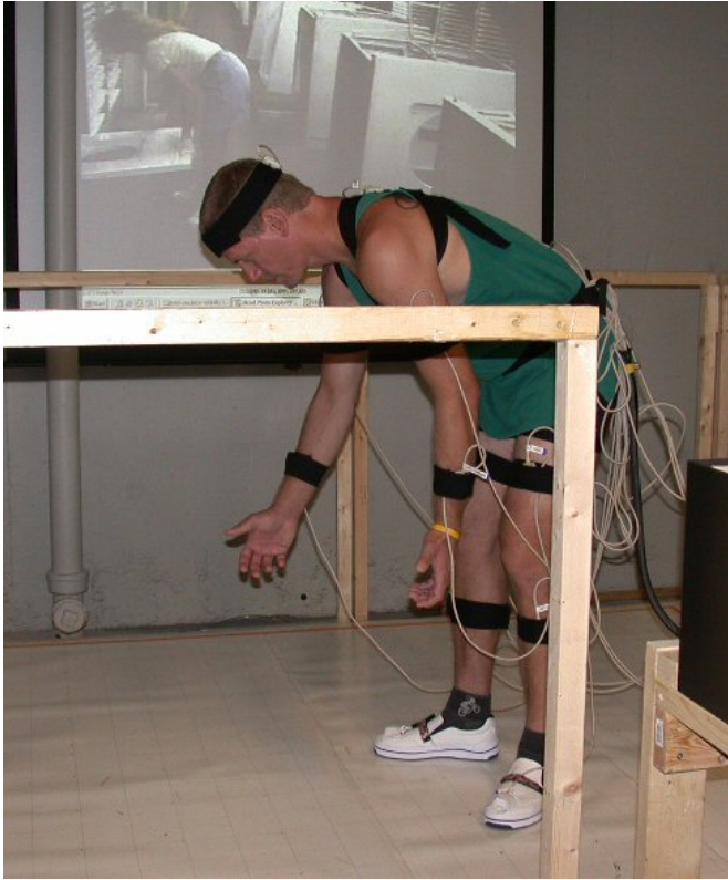
Figure 1: Instrumented “simulator” assuming a work posture on the simulation platform
