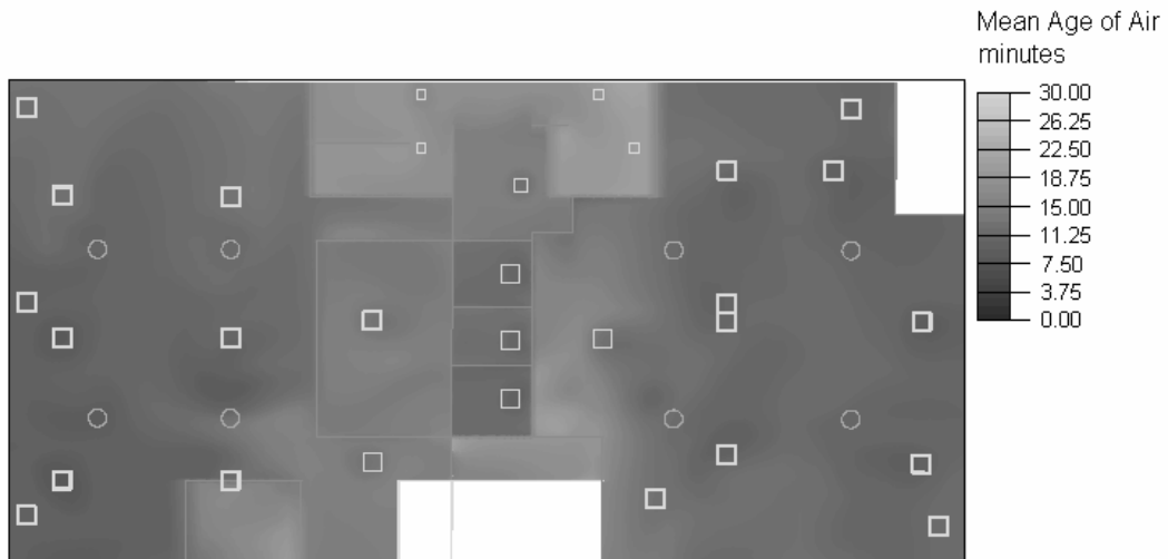
Figure 33. CFD modeling results showing mean age of air (in minutes) at three feet off the floor for the annex second floor in October 2004.
