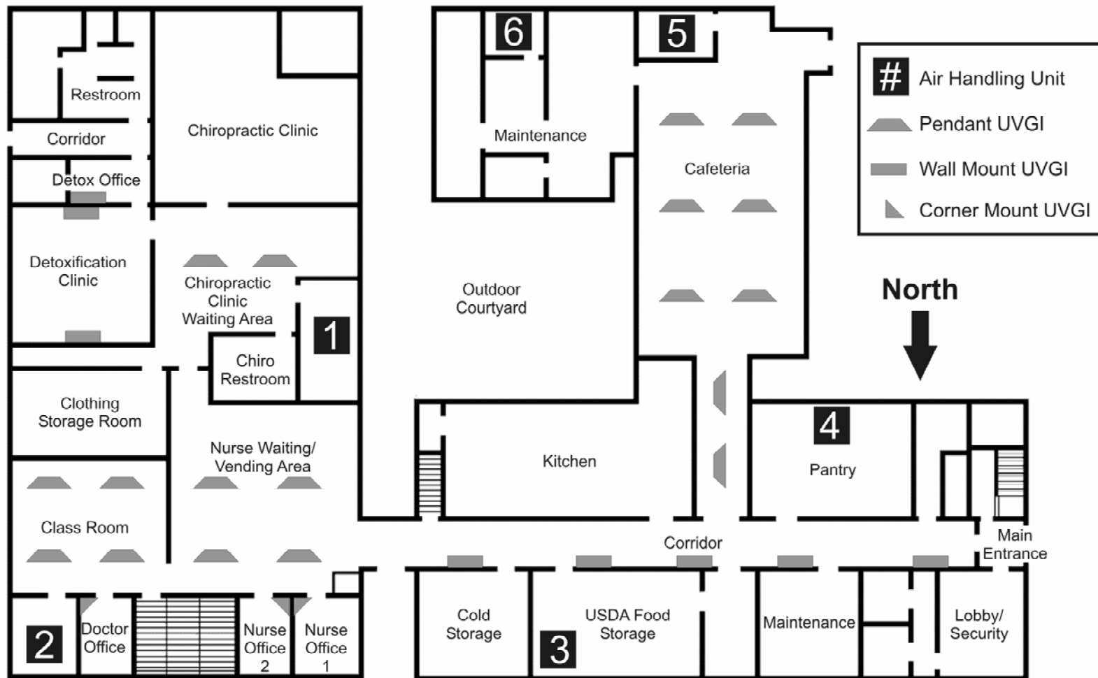
Figure 19. Placement of UVGI fixtures on the first floor of the main building.
