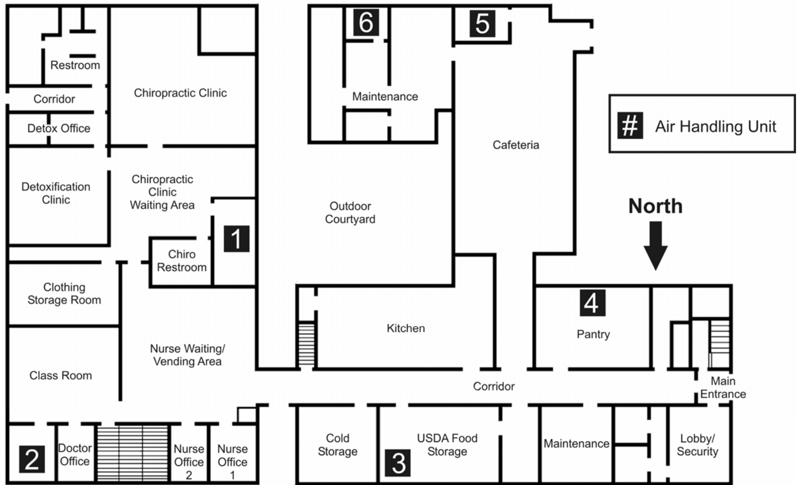
Figure 3. Basic floor plan of the main building first floor, including the locations of AHUs.
