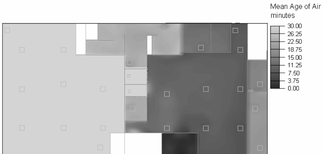
Figure 30. CFD modeling results showing mean age of air (in minutes) at three feet off the floor for the annex first floor in January 2004.
