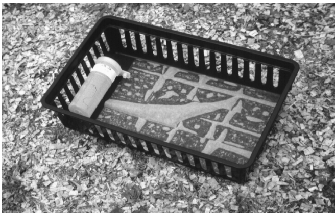
A) PbA and PbS sampling while a worker performs the dry scraping/power sanding method. B) Collection of a PbS sample with dustfall collector.
