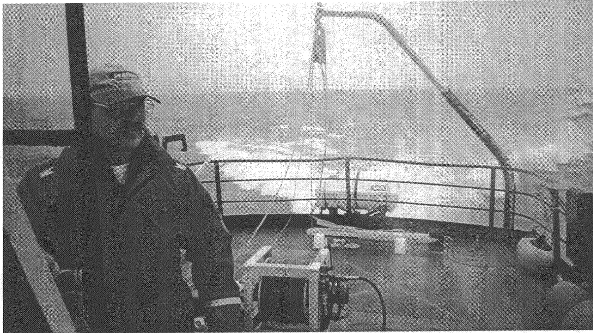
Figure 2-1. DF-1000 Tow fish and winch aboard Hickson .
