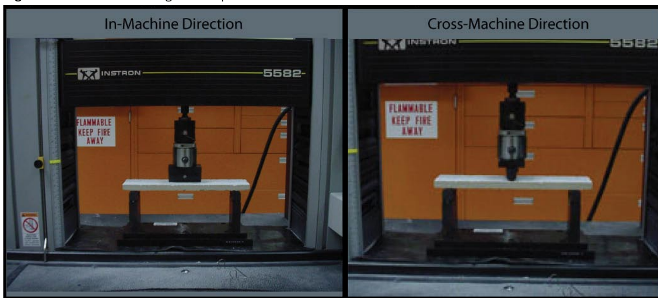
Figure 8.1: Acoustical Ceiling Tile Coupon Test
