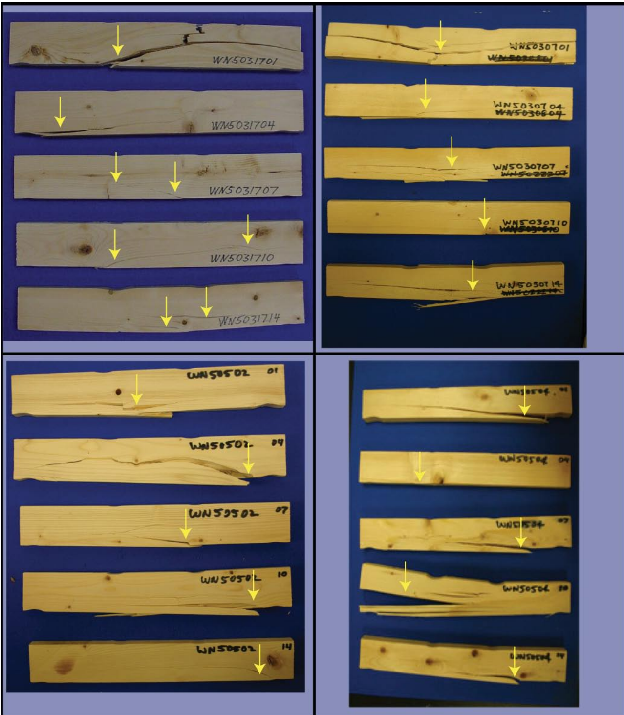
Figure C-1: Location of Break, Wood Coupons – Chlorine Dioxide Control Set
