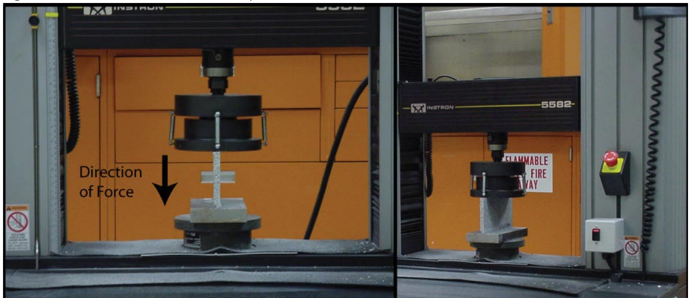
Figure 10.1: Concrete “Cinder Block” Coupon Test
