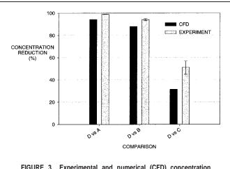
FIGURE 3. Experimental and numerical (CFD) concentration reduction for case D relative to other cases. Simultaneous 95% confidence limits are shown for the experiment.
