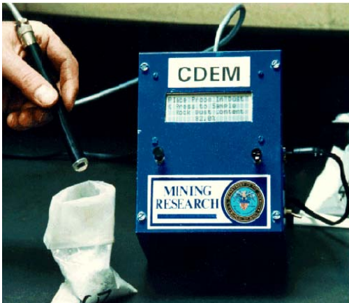
Figure 1. – The CDEM is used to analyze the composition of a coal and rock dust mixture.
