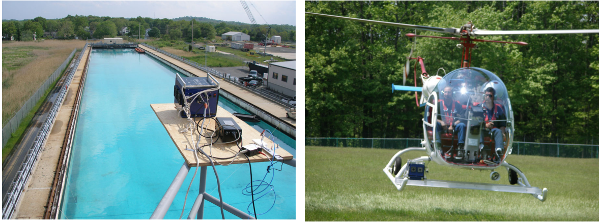
Figure 9. The DMSC imager mounted on Ohmsett tank’s crows nest (left) and on the skids of the helicopter (right).
