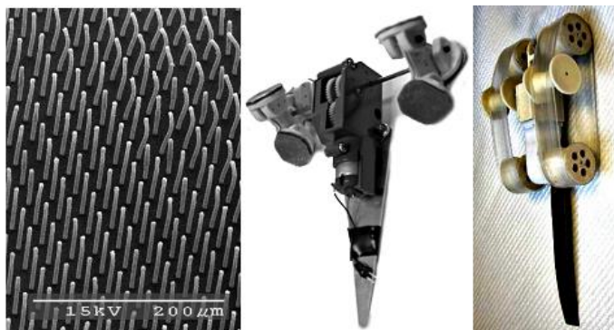
The left image shows an array of synthetic adhesive fibers 4mm in diameter that will be used to enhance the performance and robustness of climbing robots such as the ones shown in the center and right images climbing walls. Credit: Carnegie Mellon University
