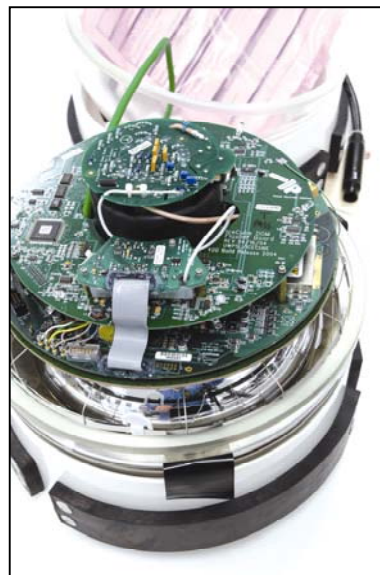
Pictured in the UW-Madison Physical Sciences Laboratory before being vacuum-sealed, each IceCube DOM is very much like a small computer. A total of 4,200 DOMs, designed to sample high-energy neutrino particles from deep space, are being deployed in 70 deep holes in the Antarctic ice.
