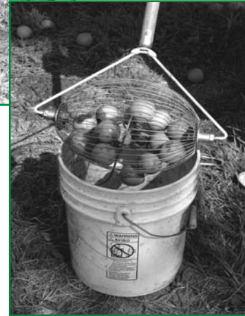
Fig. 15: (Bottom) Nuts are released from the Nut Wizard by spreading the wire cage open with a stiff wire loop
