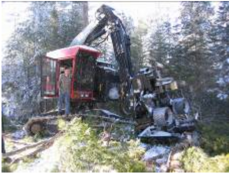
A Valmet 425 Hydrobuncher owned by A.W. Madden Inc. of Milford cuts on a Bureau of Parks and Lands lot in Bradley.
