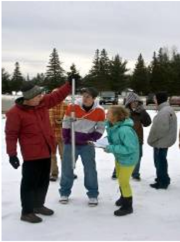
Jim Caldwell of the U.S. Geological Survey works with Mt. Abram High School students demonstrating the use of a federal snow tube to measure snow depth.
