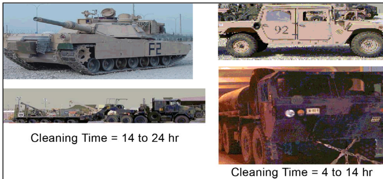
Figure 19. Cleaning times for representative vehicles (data from 886th and 887th ESFS).
