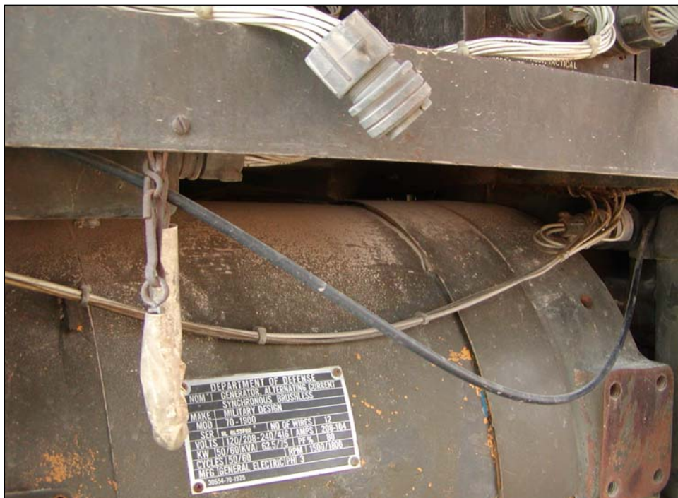
Figure 6. Soil deposits on ammunition loader.
