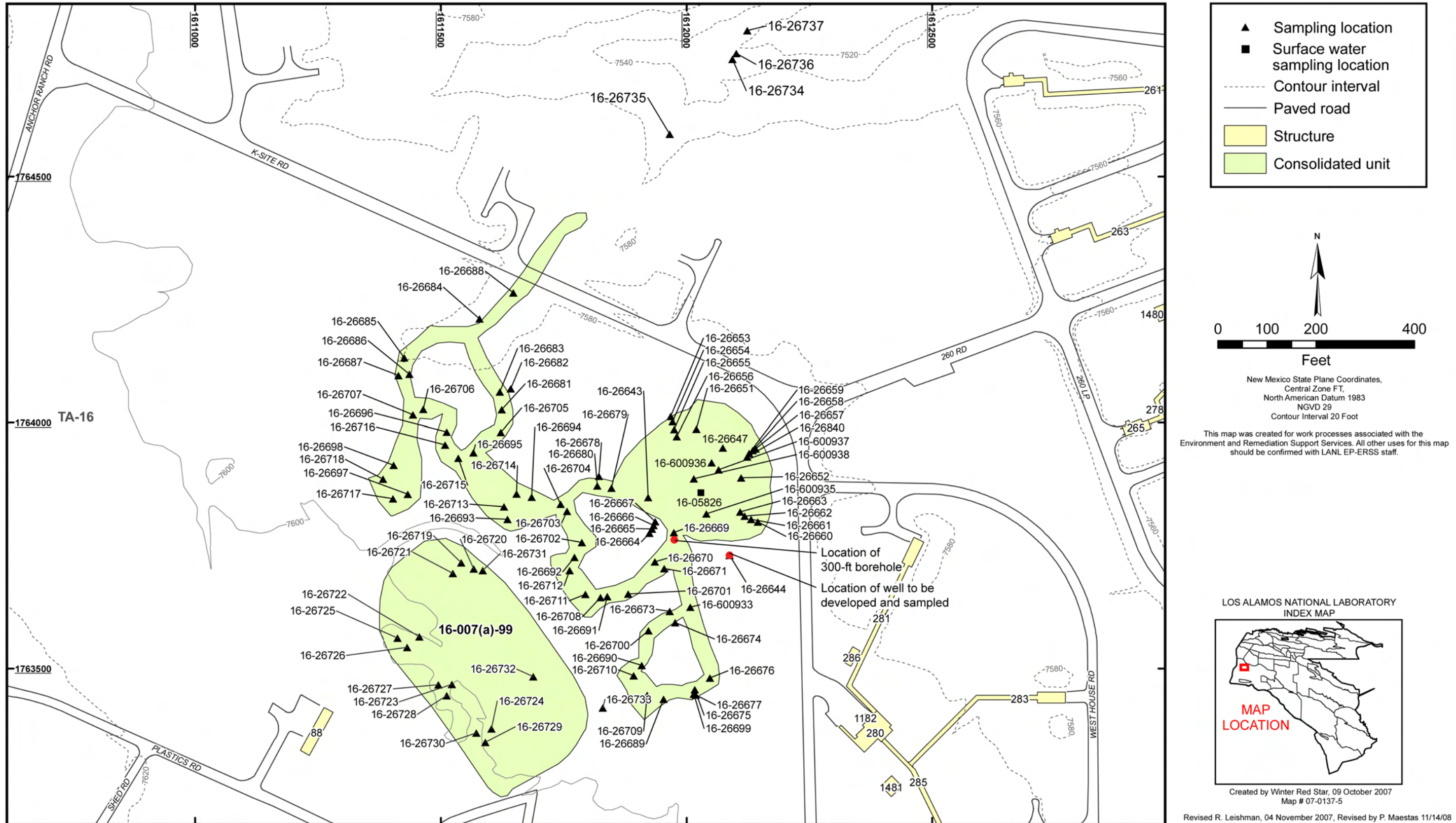
Figure 2.1-2 2006–2007 investigation sampling locations at Consolidated Units 16-007(a)-99 and 16-008(a)-99. Also shown are locations of new 300-ft borehole and well to be developed.
