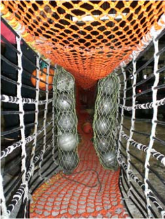
Figure 2. Bags of steel floats inside the halibut excluder.
