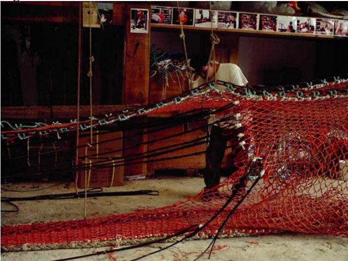
Figure 3. Halibut excluder under construction.
