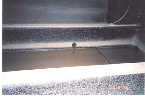
Photos 2.17 and 2.18: When ships are at even keel draft for entering the St. Lawrence Seaway, residual water is below the limber holes and is unpumpable.
