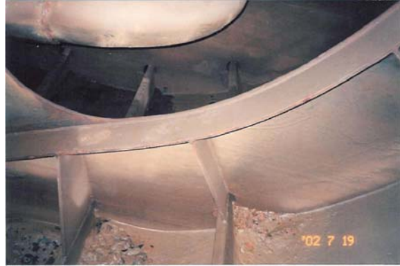
Photo 2.13: Scale, shale and sediment starting to restrict drainage where longitudinal frames pass through a bilge floor. Sediment will accumulate rapidly forward of this without remediation.
