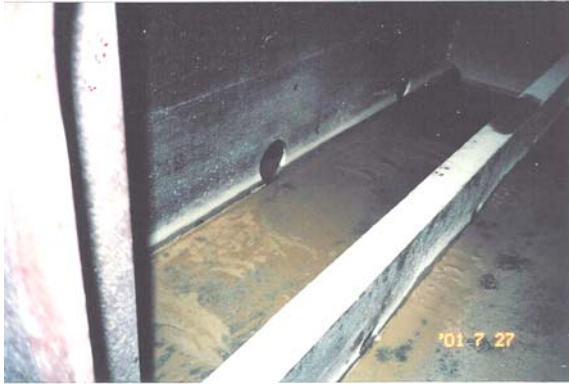
Photos 2.17 and 2.18: When ships are at even keel draft for entering the St. Lawrence Seaway, residual water is below the limber holes and is unpumpable.
