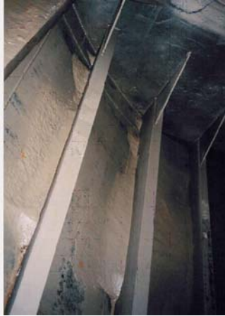
Photos 2.33 & 2.34: Sediment accumulating and compacting outboard of lower and upper framing in the bilge area, and between drainage holes in individual longitudinal frames.
