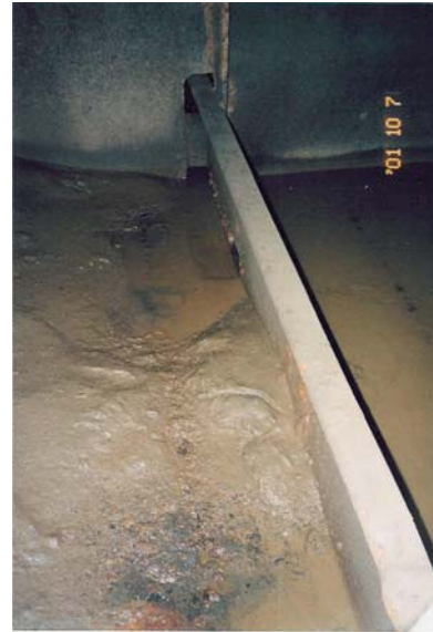
Photos 2.25 & 2.26: These sediments have accumulated and compacted outboard of bilge longitudinal and can no longer be removed by flushing
