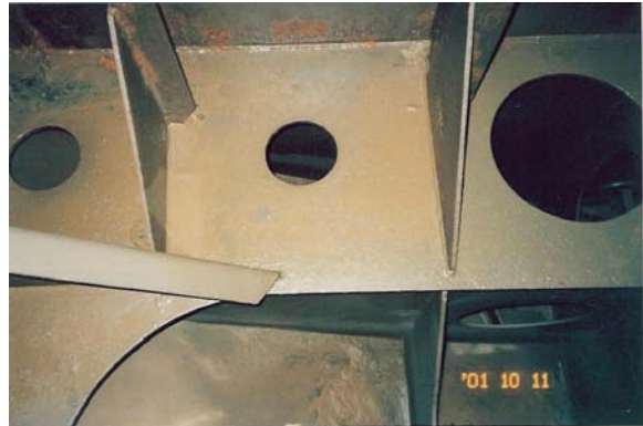
Photos 2.15 and 2.16: Sediment deposits on horizontal stringer plates within a forepeak after a single ballasting
