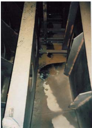
Photo 2.29 and 2.30: Deep floors and girders within a forepeak tank providing additional strength to the forefoot are particularly conducive to mud accumulations but more readily accessible for washing down.
