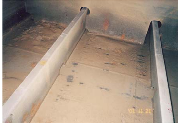
Photo 2.21: Sediment accumulation starting forward of a transverse floor and between the plane of transverse drainage through longitudinal frames.
