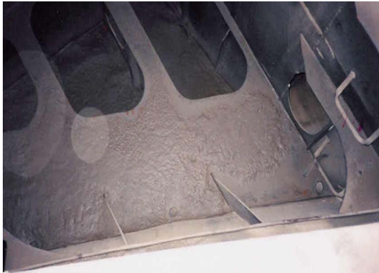
Photos 2.15 and 2.16: Sediment deposits on horizontal stringer plates within a forepeak after a single ballasting
