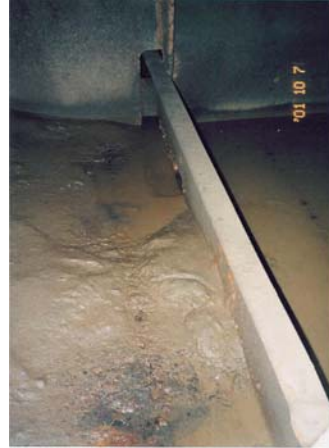
Photos 2.33 & 2.34: Sediment accumulating and compacting outboard of lower and upper framing in the bilge area, and between drainage holes in individual longitudinal frames.
