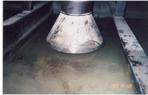
Photos 2.31 & 2.32: Longitudinal framing in a bulk carrier trading into the Great Lakes can vary in depth from 17-25 cm, and drainage to the bellmouth becomes particularly restricted once the water level in the tank drops below the top of these frames.
