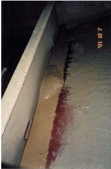
Photos 2.25 & 2.26: These sediments have accumulated and compacted outboard of bilge longitudinal and can no longer be removed by flushing
