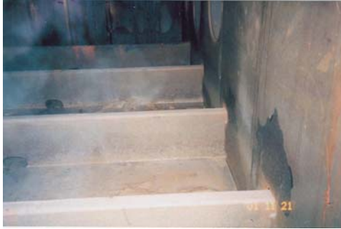
Photos 2.31 & 2.32: Longitudinal framing in a bulk carrier trading into the Great Lakes can vary in depth from 17-25 cm, and drainage to the bellmouth becomes particularly restricted once the water level in the tank drops below the top of these frames.
