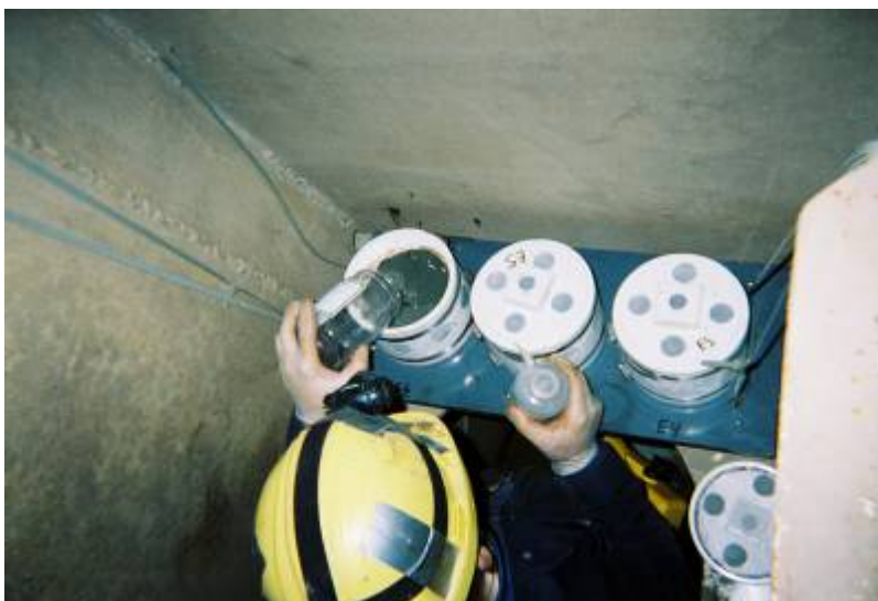
Fig. 2.25. Seeding IETraps with previously collected ballast sediments to examine effects of BWE on hatching from diapausing eggs.
