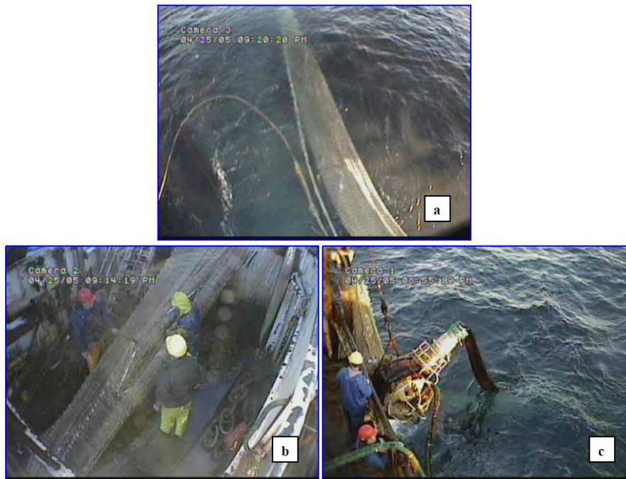
Figure 17. Example camera views from midwater trawl vessel showing net at stern (a), on the trawl deck (b) and forward starboard quarter where fish are pumped (c).
