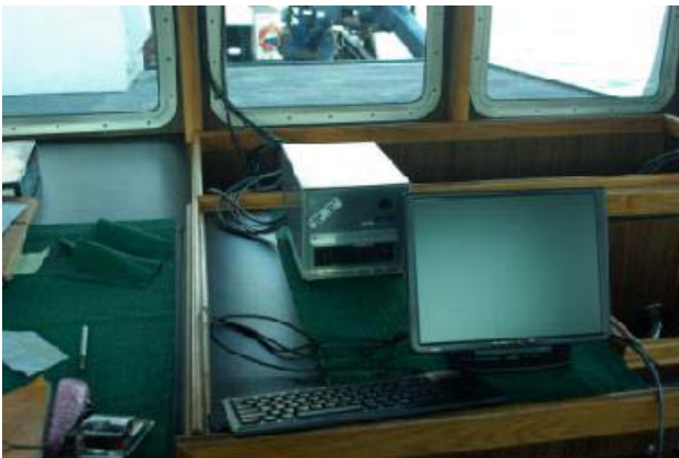
Figure A1. EM control box and user interface installations on two different vessels.
