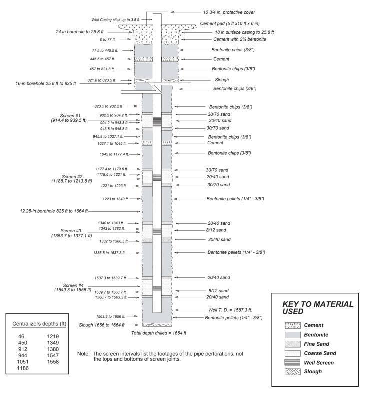
As-built well completion diagram of Well CdV-R37-2 (01/17/02).
