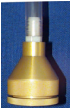
Figure 2. 102-mm and 47-mm filter holders as inverted open-face atmospheric aerosol samplers.
