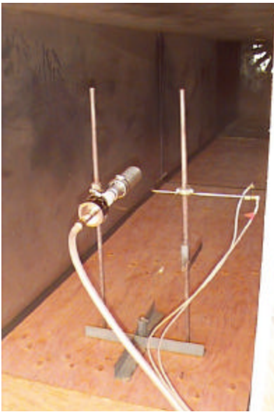
Figure 29. Shrouded probe (left) and Pitot tube (right) used to collect reference values
