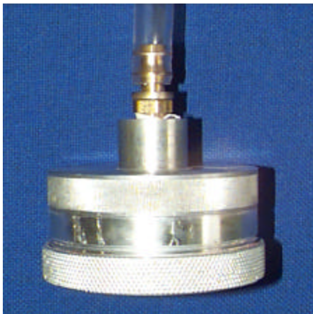
Figure 2. 102-mm and 47-mm filter holders as inverted open-face atmospheric aerosol samplers.
