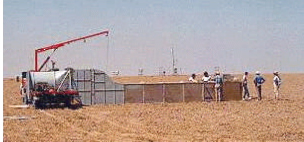
Figure 18. USDA/ARS portable wind tunnel adapted for inlet testing
