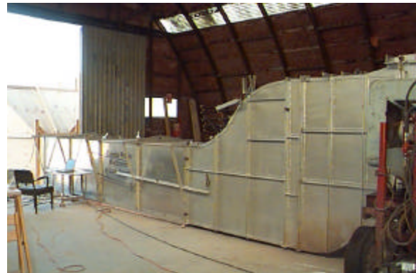
Figure 20. Tunnel transition to the ground level
