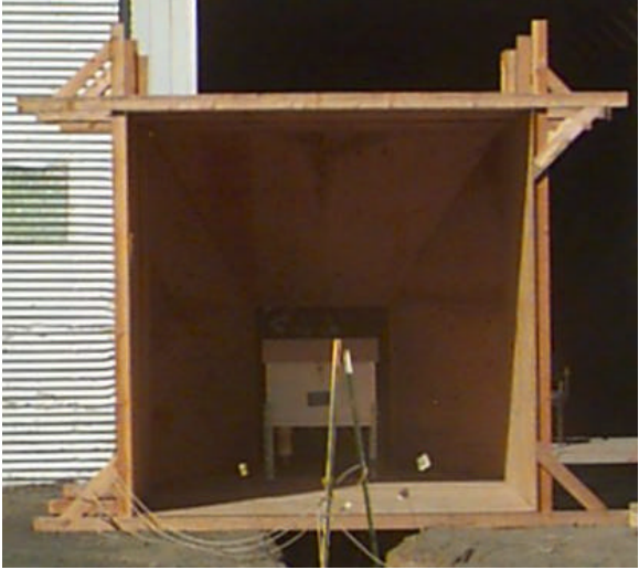
Figure 30. Test of the AIRNET sampler in the wind tunnel
