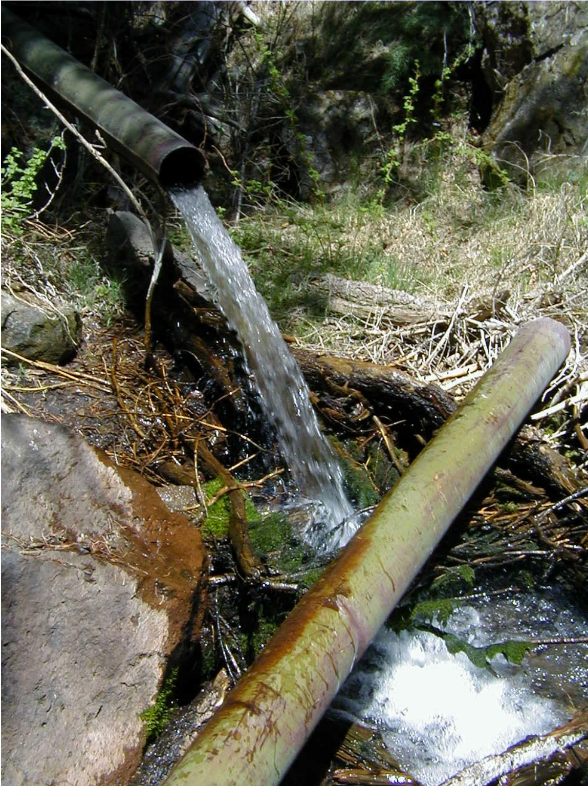
Figure E-6.2 Photograph of disconnected discharge pipe from Water Canyon Gallery taken April 27, 2000; the temperature is 14°C, and the flow rate is 120 L/min ( \pm 25\% ).
