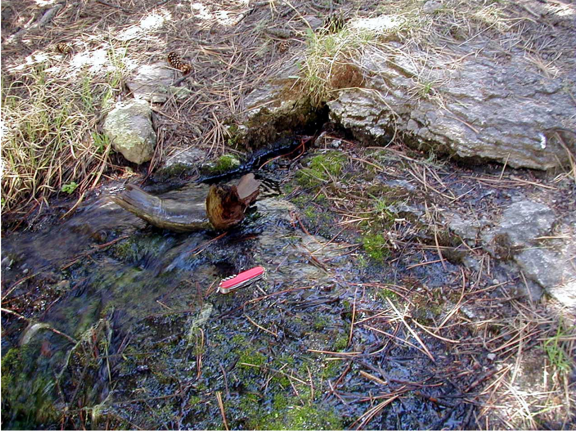
Figure E-3.1 Photograph of the largest discharge point at Seven Springs taken April 27, 2000; the temperature is 15°C, and the flow rate is 6 L/min ( \pm 10\% ). The water issues from a vertical crack in a horizontally foliated and welded Otowi Member of the Bandelier Tuff.
