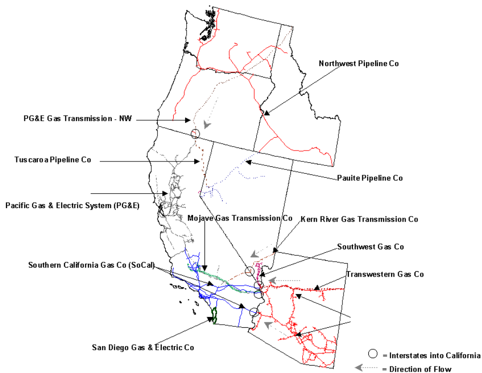
Figure 13. Major Natural Gas Pipelines Serving the Western United States
