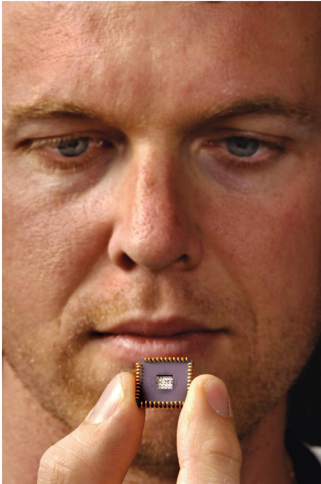
Jeb Flemming, project lead for the ElectroNeedle platform, holds a test version of the device. The prickly parts are in the center of the package. A production version could be even smaller and simpler. (Photo by Randy Montoya)
