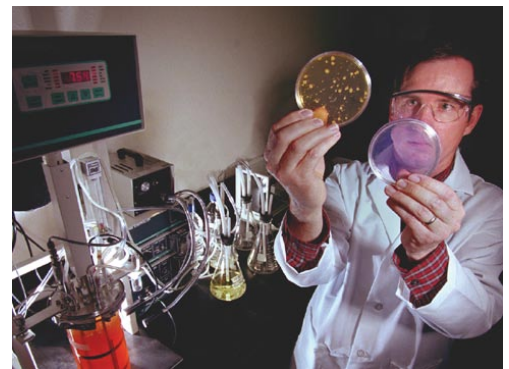
Principal Investigator Mark Tucker examines two petri dishes: one with a simulant of anthrax growing in it, the other treated with the Sandia Decon Formulation, which completely killed the simulant.
