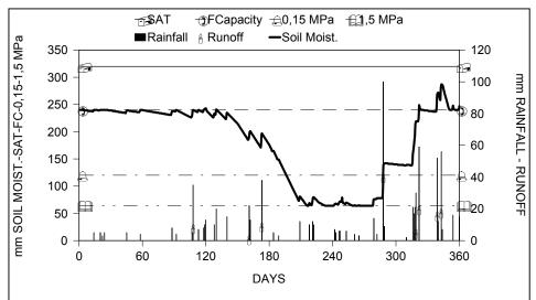
Figure 1.- Soil moisture regime in a vineyard (Mas Bernich) during 1996 (Rain above average: 760 mm. RP: 5 years). Effective soil depth: 80 cm. No surface soil sealing (Minimum water intake rate: 20 mm/h). Ksat subsoil: 0,3 mm/h
