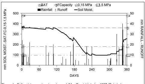
Figure 4.- Soil moisture regime in a vineyard (Mas Bernich) during 1997 (Rain below average: 483 mm. RP: 5 years). Effective soil depth: 120 cm. No surface soil sealing (Minimum intake rate: 20 mm/h). Ksat. subsoil: 0,3 mm/h
