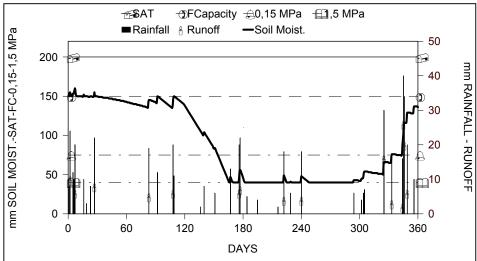
Figure 5.- Soil moisture regime in a vineyard (Mas Bernich) during the year 1997 (Rain below average: 483 mm. RP: 5 years). Effective soil depth: 50 cm. Soil surface sealing (Minimum intake rate: 4 mm/h). Ksat. subsoil: 0,3 mm/h
