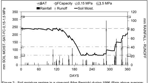
Figure 2.- Soil moisture regime in a vineyard (Mas Bernich) during 1996 (Rain above average: 760 mm. RP: 5 years). Effective soil depth: 80cm. Surface soil sealing (Minimum intake rate: 4 mm/h). Ksat. subsoil: 0,3 mm/h
