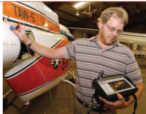
Kirk Rackow looks for cracks on the tail section of a retired helicopter using a nondestructive inspection device called an eddy current sensor.
