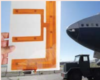
In situ sensors can be mounted on an aircraft structure.
