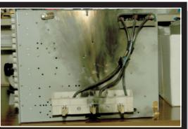
Left: Facility employee assisting in the investigation shows front of motor control center bucket where arc occurred. Above: Burn marks are evident on the back side of the bucket where self-tapping screw contacted terminal block.
