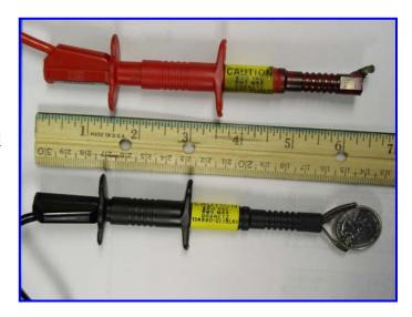
transformer, a short occurred between the secondary and primary lugs causing half of the metal teeth of one probe to vaporize, and trip the circuit breaker on the primary side of the transformer. The open breaker caused a conditioned power loss to twelve laboratory rooms.
