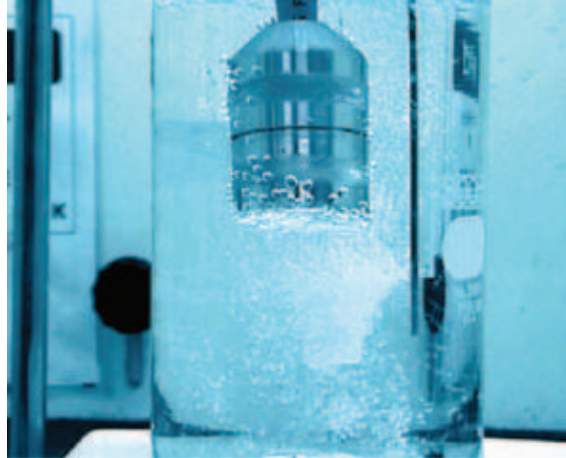
Sandia-developed micro-chemical sensors, called chemiresistors, operate underwater to detect and measure volatile organic compounds.
