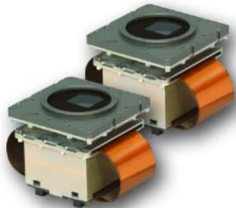
This Sandia satellite-based optical sensor package, only 1.5 cubic inches, provides a revolutionary level of processing. Sensing and signal processing are done at the equivalent speed of more than a gigabit per second, a level never before approached in a package this small.
