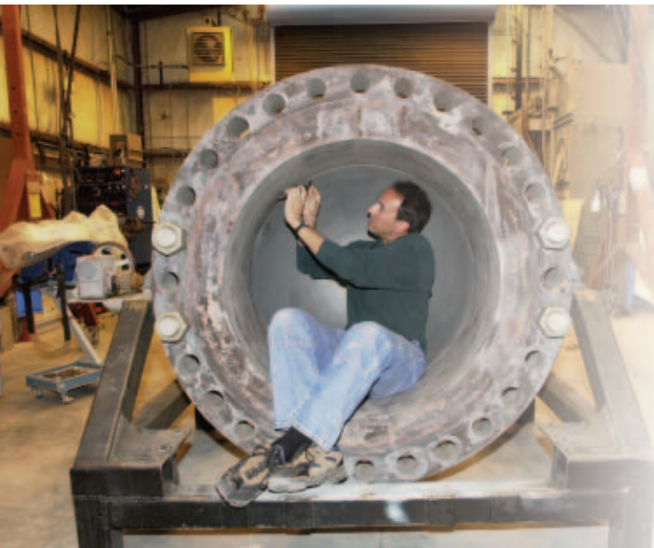
Richard Simpson of Sandia's Applied Nuclear Technologies department measures a weld in a 1/5-scale-model pressure vessel lower head assembly.
