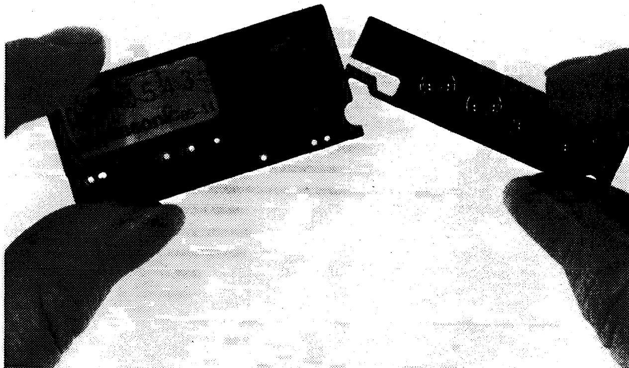
Figure 26. Construction of a typical Panasonic dosimeter.
