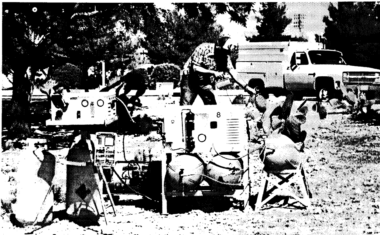
Figure 10. EPA Monitoring Technician Surveys Ambient Environmental Radiation Using a Handheld Survey Instrument. Foreground from left to right: constant flow air sampler, gamma exposure-rate recorder, and compressed noble gas sampler.
