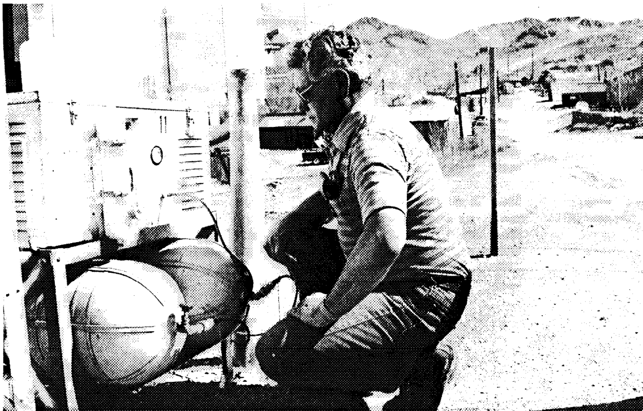
Figure 15. EPA Monitoring Technician Changes Noble Gas Tanks and Checks Gauges at Community Monitoring Station.
