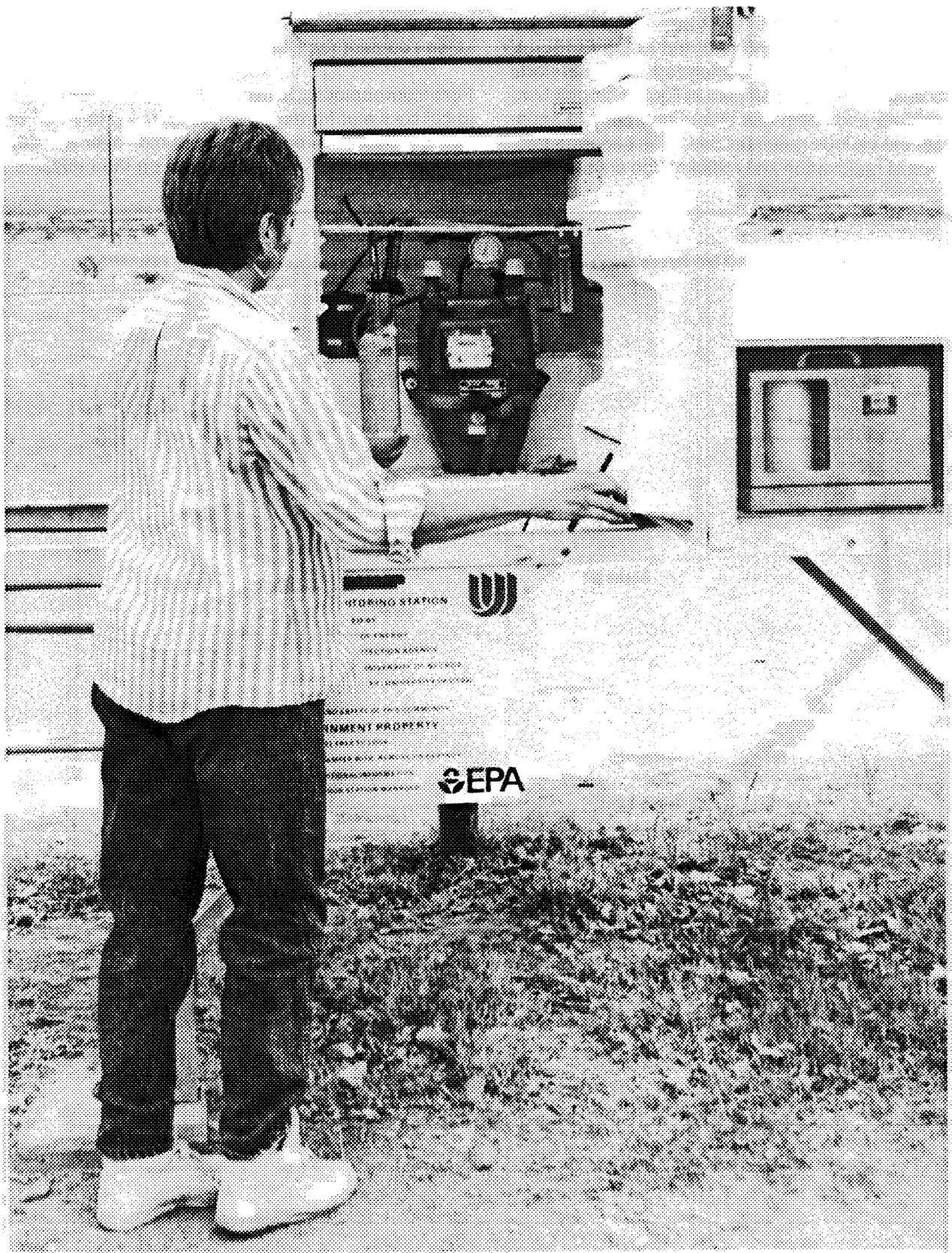
Figure 17. EPA Monitoring Technician Changes Molecular Sieve on Tritium Air Sampler at Community Monitoring Station.
