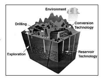
systems; drilling, reservoir testing, and modeling optimize production and predict useful lifetime; steam turbines use natural steam or hot water flashed to steam to produce electricity; binary conversion systems produce electricity from water not hot enough to flash.
