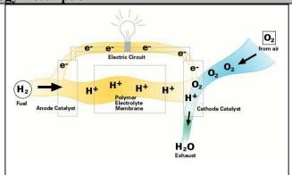
presence of a catalyst. Ions are conducted through the electrolyte while the electrons flow through the anode and the cathode via an external circuit. The current produced can be utilized for electricity. The ions and electrons then recombine, with water and heat as the only byproducts.
