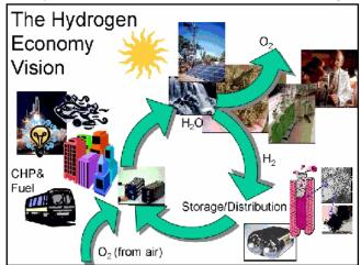
the hydrogen to power a fuel cell, internal combustion engine, or turbine, where hydrogen and oxygen (from air) recombine to produce electrical energy, heat, and water to complete the cycle. This process produces no particulate matter, no carbon dioxide, and no pollution.
