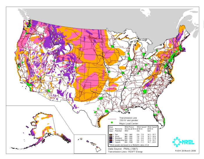
Figure 13.7. Wind Resources, Transmission, and Load Centers
