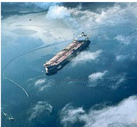
Exxon Valdez tanker encircled with a containment boom. (Photo credit: Exxon Valdez Oil Spill Trustee Council)
