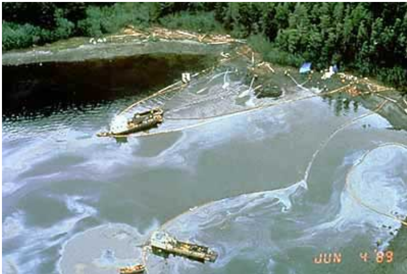
A brown sediment plume and sheens of refloat oil drift away from this oiled beach as it is cleaned by a team applying high-pressure, hot-water washing. Refloating of oil and the release of sediments are often unavoidable consequences of shoreline cleanup that can cause additional environmental harm. (Photo credit: OR&R, NOAA)
