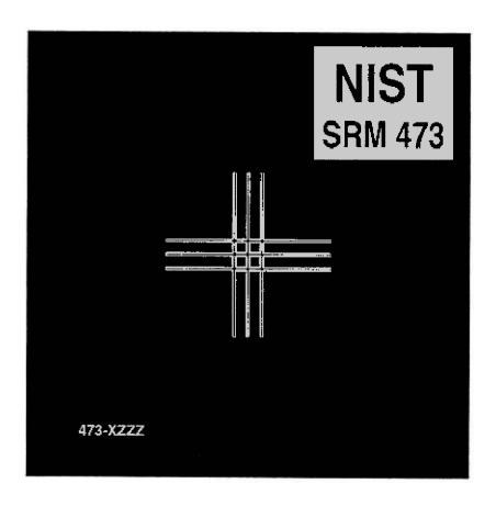
Figure 1. A view of the overall pattern on SRM 473. The basic measurement pattern is repeated eight times about the center. The horizontal and vertical lines help locate the patterns.
