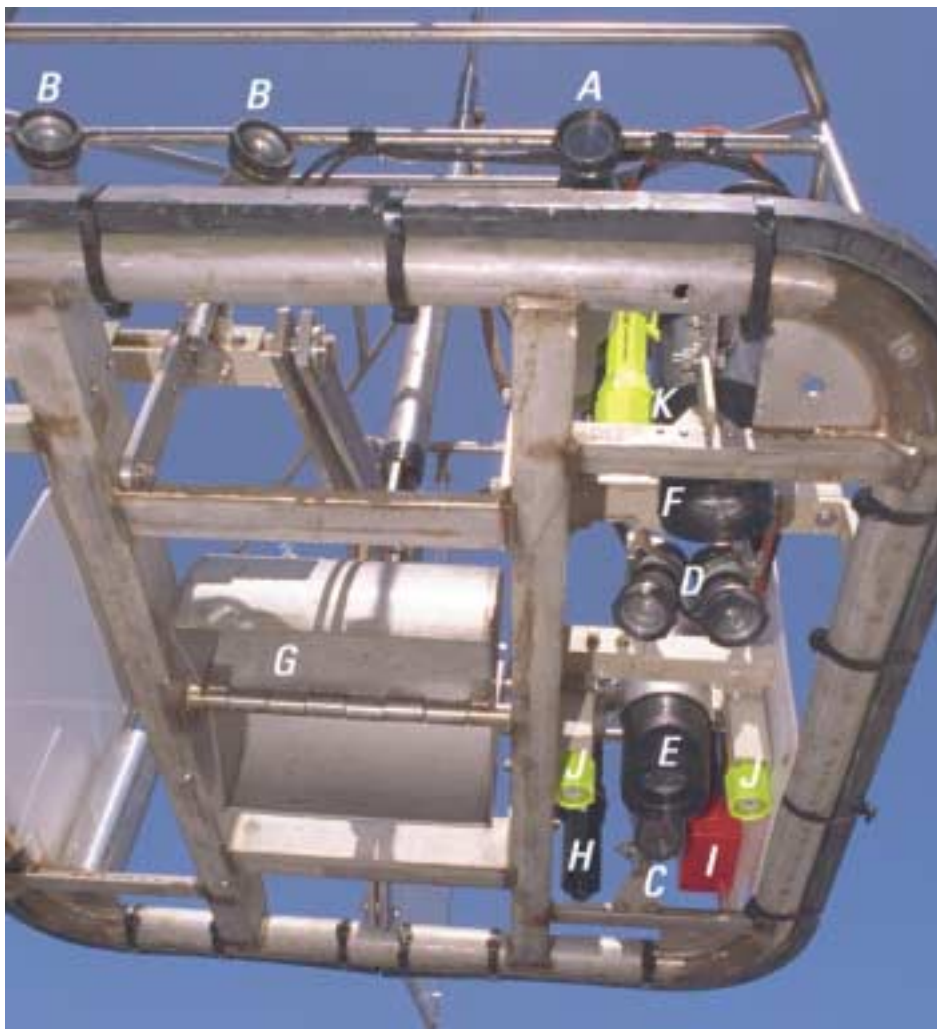
Figure 1. A view of the SEABOSS from below (with base plates removed; see fig. 2). Photograph by Dann Blackwood, USGS. The instruments are as labeled: A, forward-looking video camera; B, lights for forward-looking video camera; C, downward-looking video camera; D, lights for downward-looking video camera; E, 35-millimeter still camera; F, strobe light for still camera; G, modified Van Veen grab sampler; H, depth sensor; I, junction box; J, parallel lasers for scale; K, angled laser for range.
