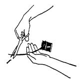
Next, attach one end of each wire to one of the motor's outlets. Tape the wires to the molding, at the end without the motor. Attach the other two ends of the wire to a :voltmeter.
