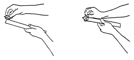
Second, cut two 3O-cm pieces of electrical connecting wire. With a pair of scissors, take off 2 cm of rubber insulation from both ends of the two wires. Do this by pinching softly with the scissors on the rubber casing, cutting it slightly; then pull the scissors towards the wire's end, pulling off the casing.
