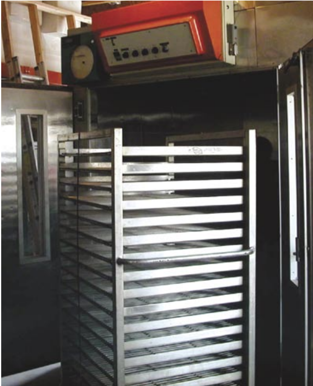
The meat, racked and loaded onto trucks, is now ready for processing in the Koma 4000 brand smoker.
