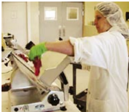
Power meat slicers are part of the quality control process. They ensure that every slice of meat has the uniform thickness essential for consistent drying.
