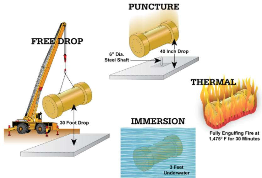
To be certified by the Nuclear Regulatory Commission, every type of transportation cask must be able to withstand all of the tests shown above.
