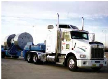
A legal-weight truck carries a cask containing spent nuclear fuel. Drivers are specially trained and certified, must be accompanied by at least one escort, must report in with the DOE every two hours, and are continuously monitored and tracked by satellite.
