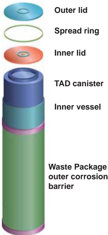
*In the “canister within a canister” approach, three containers are nested inside one another to safely shield the radioactive waste.*
