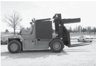
A Specially Designed Shielded Forklift will be Used to Transport Debris to the Remote-Handled Facility for Processing at West Valley .
